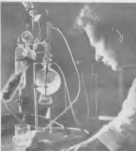
KJELDAHL APPARATUS, above, is used to determine nitrogen in petroleum fractions. The infrared cell, right, determines the nature of hydrocarbon molecules which adhere to a catalyst surface.
